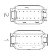
Figure 18: Connector numbering and placement CCpilot V510/710.
