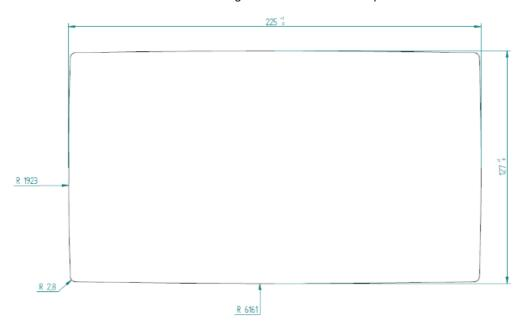
Figure 11: Panel cut-out CCpilot V710
