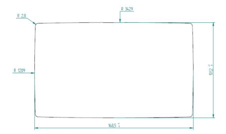
Figure 10: Panel cut-out CCpilot V510
