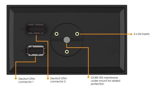
Figure 5: CCpilot V710 rear side view
