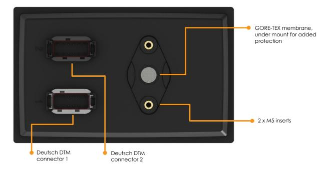
Figure 4 CCpilot V510 rear side view
